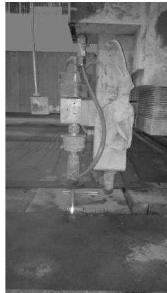
Fig.2. Illustration of AWJM operations
