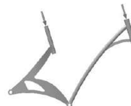
Fig.5. First frame loads
