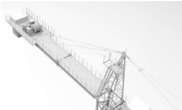
Fig.6. Counter-jig of the tower crane
