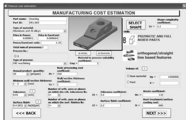
Fig.4. Representation of the applied software for the estimation of housing manufacturing cost for variant 1
