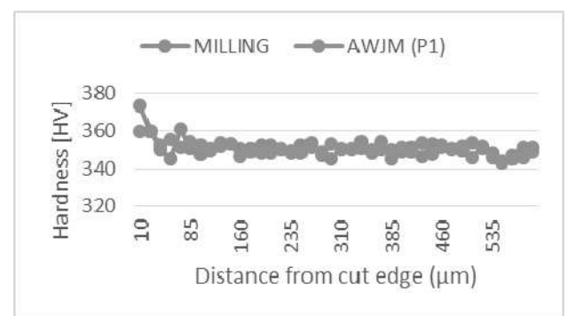
Fig.6. Micro hardness results of AWJM (P1) and Milling.
