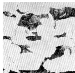
Fig. 12. 18 MnCr 10 steel structure, hot-rolled. R_m = 570 MPa. Elongation at fracture 22%. Structure: ferrite and perlite, banded structure. Inadequate quality of the cutted surface, with traces of impurities carried in from the hot-rolled surface. Low edge endurance.
