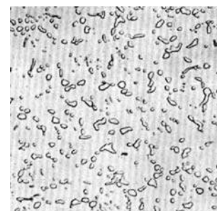
Fig. 11. OLC 45 steel structure, annealed, special for fine blanking. R_m = 400 MPa. Elongation at fracture 35%. Structure: spheroidal cementite, equally dispersed. The best quality of the cutted surface, even for complicated shape parts. Maximum edge endurance.
