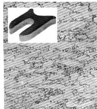
Fig.2. Blanked edges very smooth. Material: C=0,36%, Si=0,27%, Mn=0,61%, P=0,018%, S=0,031%. Tensile strength 490 MPa. Structure: well transformed spherical cementite. Hot-rolled with further heat treatment.
