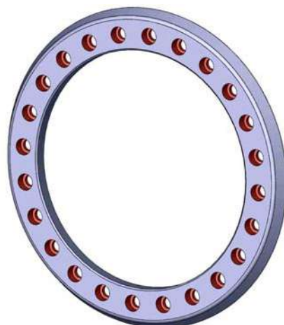
Sl. 4 Pritezni prsten zapornog tela LZ DN 700 (3D model)
